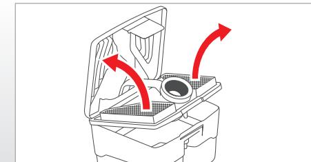
Replacing the special hygiene filter and special hygiene prefilter
