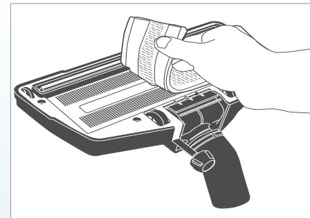
**ⓘ** A dirty microfibre pad can be cleaned by hand or in a washing machine at max. 60°C. Do not use fabric softener.
