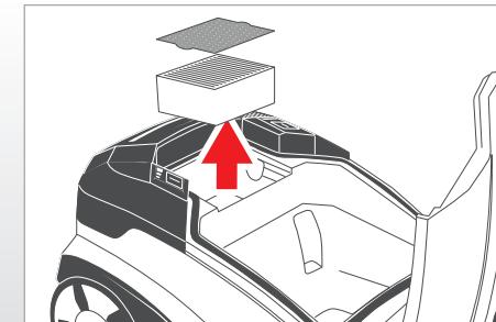
Replacing the exhaust filter
