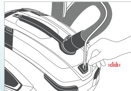
Connect the correct end of the telescopic wand to the handle of the suction hose and connect the spray nozzle to the telescopic wand.
